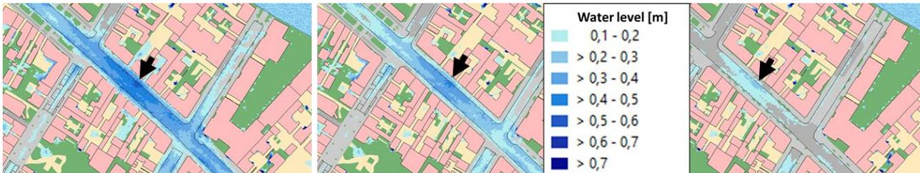
**Figure 2.** Maximum water levels in the centre of flooding with rainfall load R1. From left to right: base model, swales (sized to T = 100 a): degree of Implementation 50 % and 100 %
